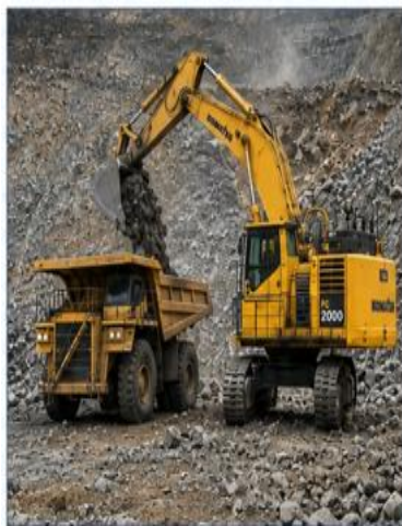
Fig. 1. Excavator-truck complex in an open-pit mine
