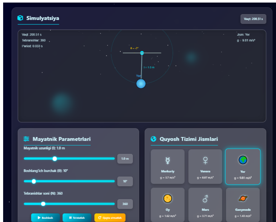
Figure 2. A model for determining the acceleration of free fall in a virtual laboratory using a mathematical pendulum.
