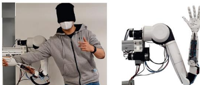
Figure 3: ( a ) The proposed humanlike arm hand system for DB communication with t-ASL[19], ( b ) blindfolded human who is unfamiliar with ASL [19]
