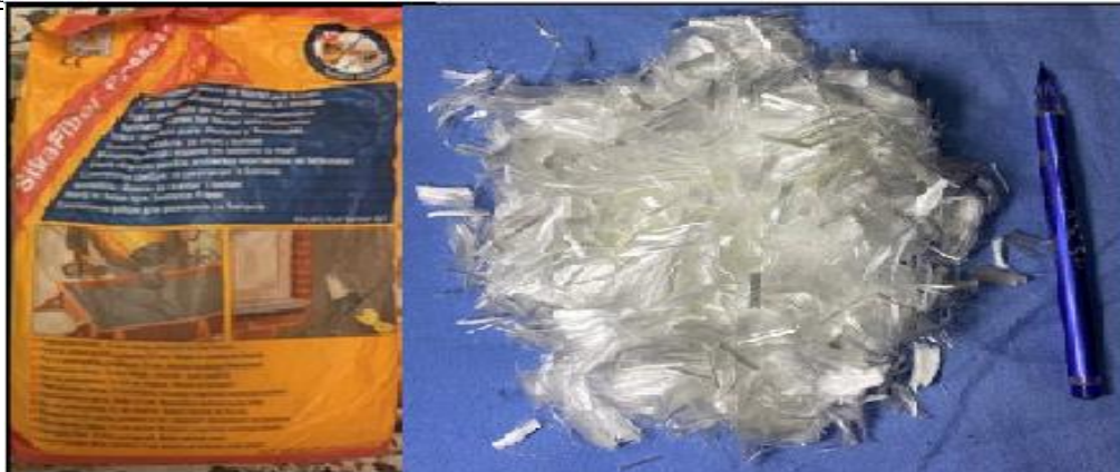
Plate 2: Polypropylene fiber (PPF) used in the present research
